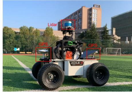
Fig. 1. The Ackermann-steering vehicle.
